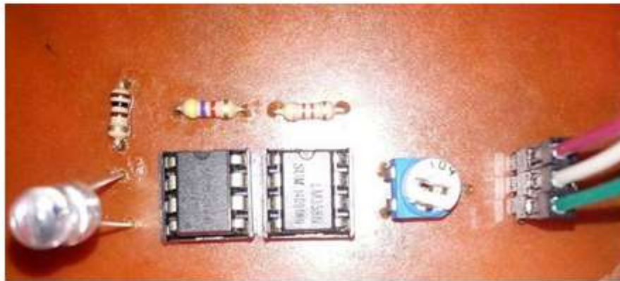
Figure 10. Components soldered on receiver PCB
